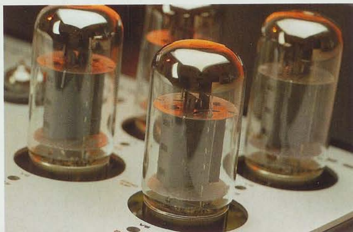
6550s [right] take on output duties; the 6N1Ps [below] have damping rings; reservoir capacitors are by Nichicon
