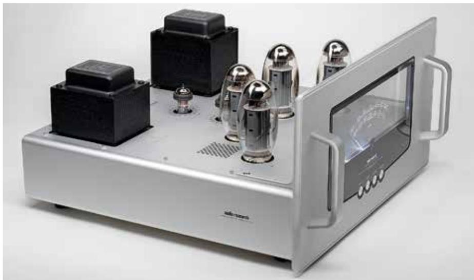
**ABOVE:** Factory-matched and held in check by ARC's auto-bias regime, the two pairs of KT150 tubes are fan-cooled once the lid is in place. Two custom-made transformers are fitted – one for the PSU with three secondaries [furthest] and the other with two primaries and three speaker output taps
