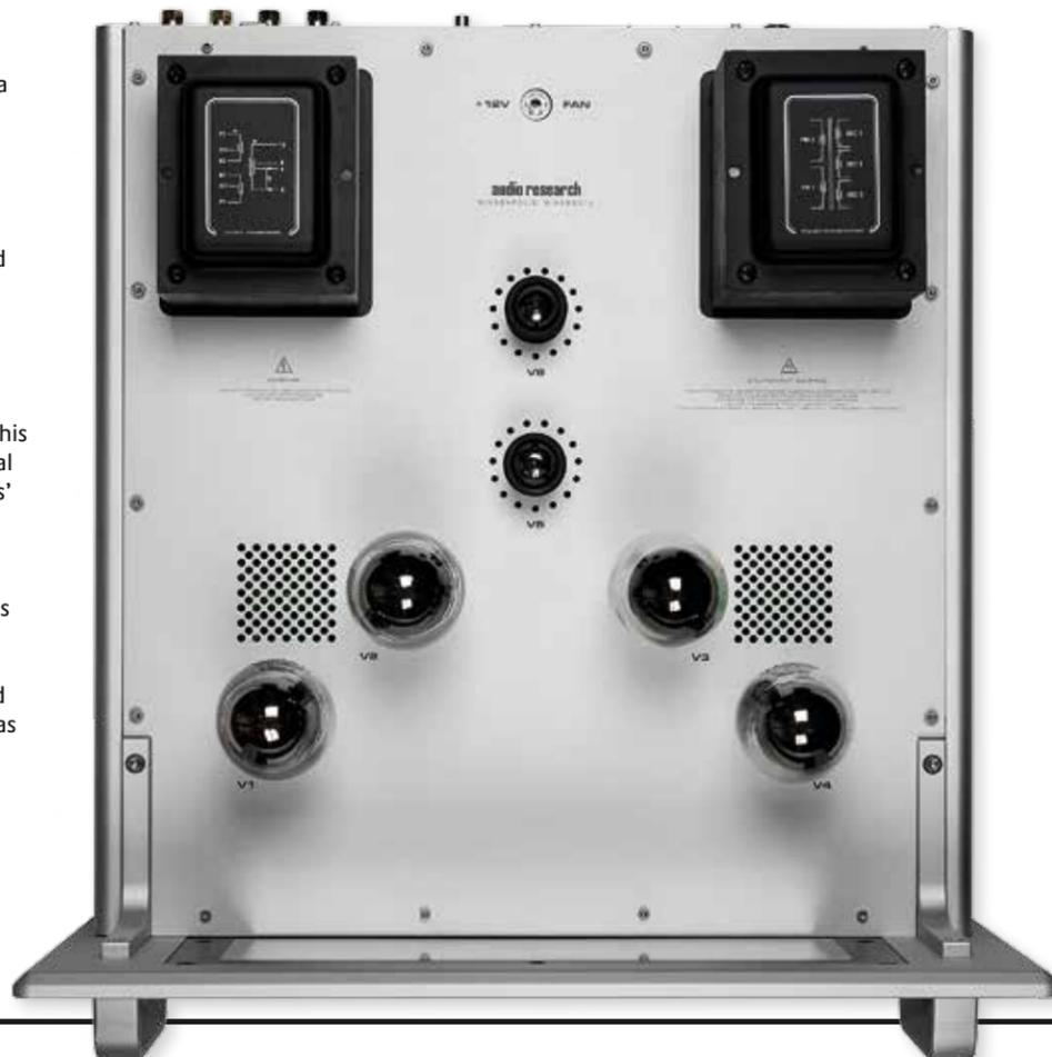
**RIGHT:** Cover (and integral fan) removed reveals the two 6H30 driver triodes and quad set of KT150 output tubes. Auto-biasing will also accommodate lower output 6550, KT88, and KT120 tubes
