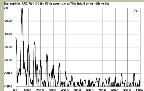
Fig.11 Audio Research Reference 110, 8 ohm tap, spectrum of 50Hz sine wave, DC–1kHz, at 70W into 8 ohms (linear frequency scale).
