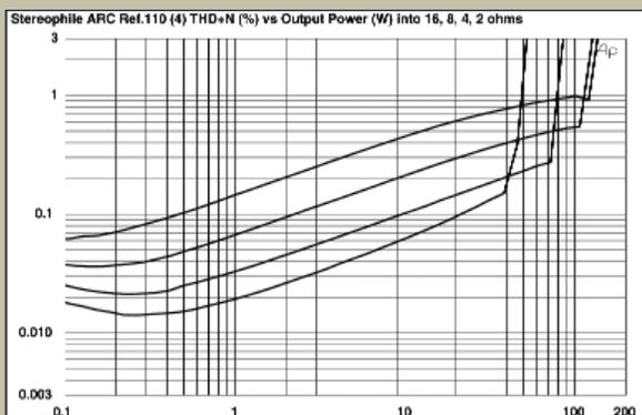
Fig.4 Audio Research Reference 110, 4 ohm tap, distortion (%) vs 1kHz continuous output power into (from bottom to top at 10W): 16, 8, 4, 2 ohms.
