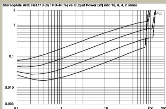
Fig.5 Audio Research Reference 110, 8 ohm tap, distortion (%) vs 1kHz continuous output power into (from bottom to top at 10W): 16, 8, 4, 2 ohms.
