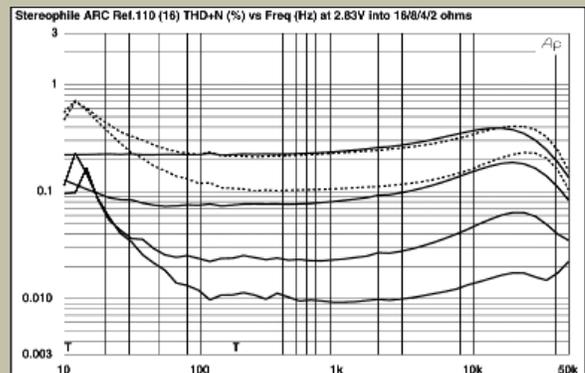
Fig.9 Audio Research Reference 110, 16 ohm tap, THD+N (%) vs frequency at 2.83V into (from bottom to top): 16, 8, 4, 2 ohms (right channel dashed).
