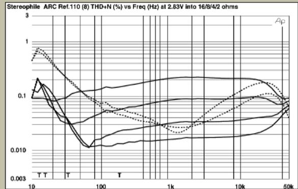
Fig.8 Audio Research Reference 110, 8 ohm tap, THD+N (%) vs frequency at 2.83V into (from bottom to top): 16, 8, 4, 2 ohms (right channel dashed).
