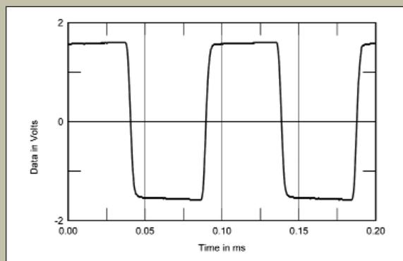
Fig.2 Audio Research Reference 110, 8 ohm tap, small-signal 10kHz squarewave into 8 ohms.
