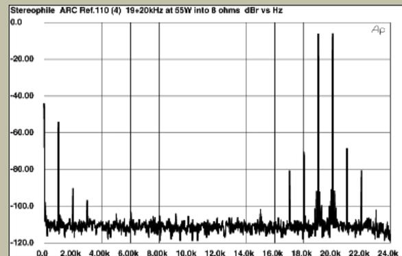
Fig.12 Audio Research Reference 110, 4 ohm tap, HF intermodulation spectrum, DC–24kHz, 19+20kHz at 55W peak into 8 ohms (linear frequency scale).
