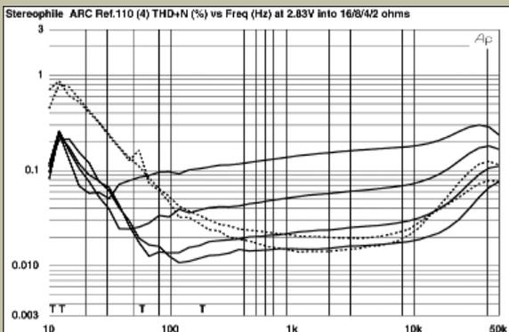
Fig.7 Audio Research Reference 110, 4 ohm tap, THD+N (%) vs frequency at 2.83V into (from bottom to top): 16, 8, 4, 2 ohms (right channel dashed).
