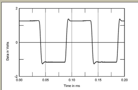
Fig.3 Audio Research Reference 110, 4 ohm tap, small-signal 10kHz squarewave into 8 ohms.
