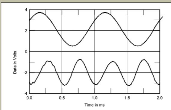
Fig.10 Audio Research Reference 110, 4 ohm tap, 1kHz waveform at 1.5W into 8 ohms (top), 0.039% THD+N; distortion and noise waveform with fundamental notched out (bottom, not to scale).
