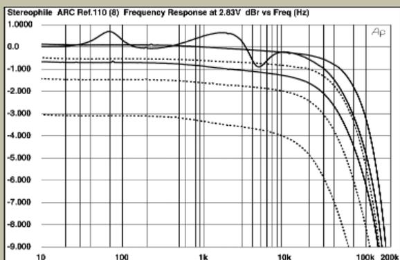
Fig.1 Audio Research Reference 110, 8 ohm tap, frequency response at 2.83V into (from top to bottom at 2kHz): simulated loudspeaker load, 8, 4, 2 ohms (1dB/vertical div., right channel dashed).
