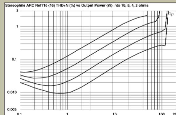
Fig.6 Audio Research Reference 110, 16 ohm tap, distortion (%) vs 1kHz continuous output power into (from bottom to top at 10W): 16, 8, 4, 2 ohms.
