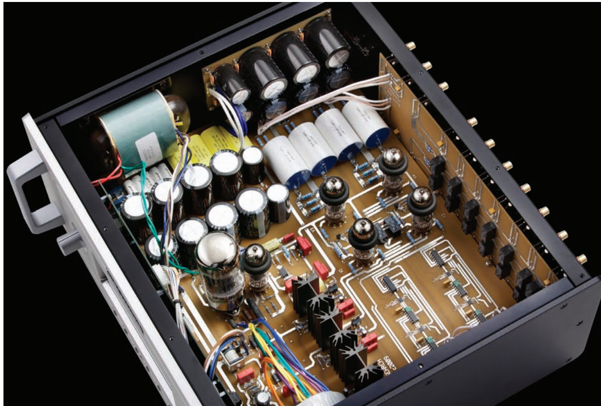
The Ref 5SE's interior is stuffed to the gills with capacitors.
