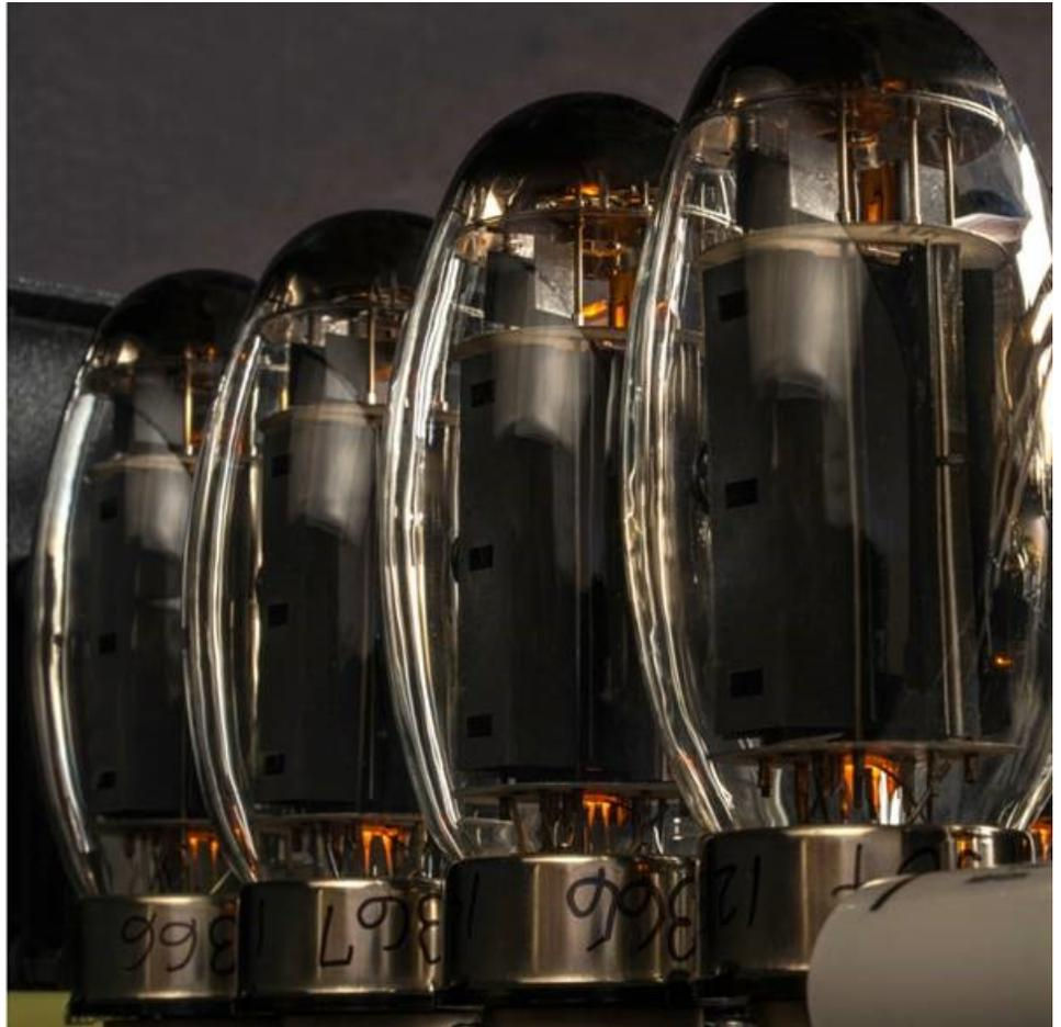
As to why: There's a lot of mass in most tube amps; the chassis, transformers and circuitry all need to reach thermal equilibrium. Reaching operating temperature stability allows the circuit to achieve maximum electrical stability which minimizes distortion characteristics.
